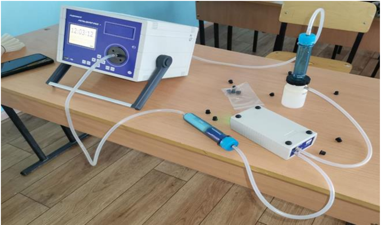
Figure 3. Scheme of sample measurement. Radon in water
