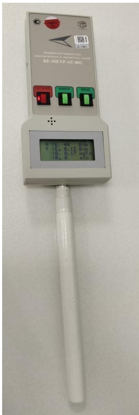
Figure 14 "VE-METER-AT-002" Meter parameters electric and magnetic fields
